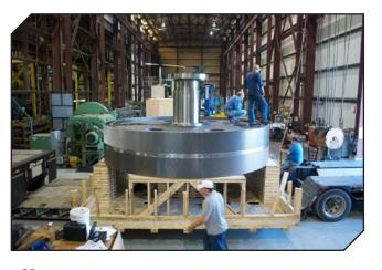
ring and/or hub center section, welded together with structural or forged plate center sections. The lack of quality casting vendors has sent us down this path.
