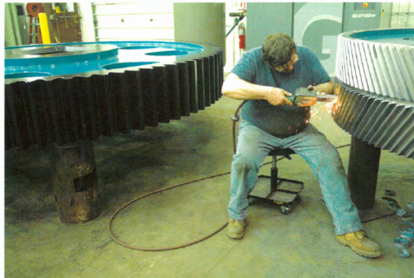
Melton Stilwell polishes the roots of a gear in the preparation and handling area at HMC in Princeton, Ind. HMC manufactures large gears and does custom machining.
